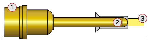
Equip-Test Spring Loaded Probe connects to DUT Terminal
